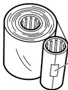
Remove the label of the lamination film and place on it to the surface of the winding bobbin.
