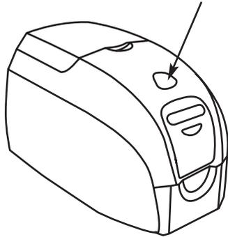
Open printer lid by pressing the cover release button on the top of your printer.
