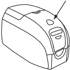
Open printer lid by pressing the cover release button on the top of your printer.
