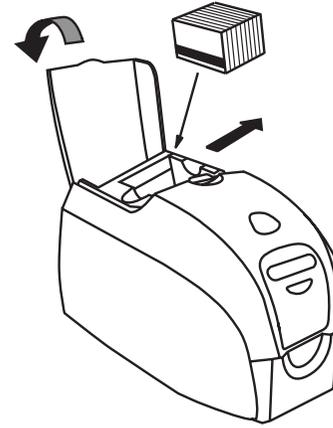
Open card feeder cover. Slide card guide all the way to the right until it locks in place with an audible click.
