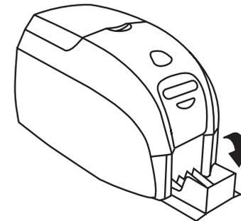
Raise the printer lid and rotate the hopper down.
