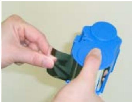
Install a fresh cleaning cassette by locating the rectangular pin on the cleaning mechanism in the receptacle on the cassette. Push the cassette gently home, ensuring that the internal grooves on the upper spool engage the teeth on the takeup drive.
