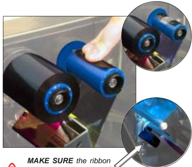
**MAKE SURE** the ribbon is **between** the arms of the ribbon sensor left of the printhead.
