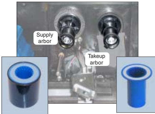
**P640i color ribbon**, left, and empty core, right. The flange end with internal grooves goes to the back.
