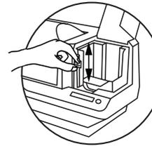
This item can be operated to set the card thickness and to prevent more than one card feeding into the printer at the same time.
