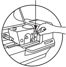
The card cleaning cartridge is packed separately from the printer in a protective plastic bag. Remove carefully and peel off tape. A loud 'CLICK' will indicate the cartridge is correctly installed.
