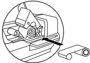
Turn on the power and raise the printhead. Load ribbon onto the supply and take-up spindles. Lock the printhead down.
